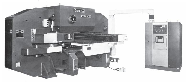
This 30 ton Vela II Amada Machine shapes and perforates our side panels with computer directed programming accurate to + .001".
