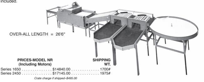
An example of how our well engineered units fit together to produce a complete tomato packing machine. Notice use of our waxer, sizing units fitted with rubber sizing belts and side delivery conveyors.
