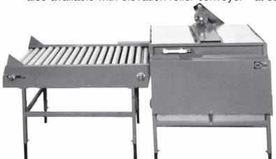
OVER-ALL LENGTH = 9' ONE 1/2 HP MOTOR AND ONE 1/4 HP GEARMOTOR RUN MACHINE
